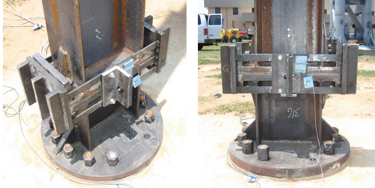
Figure 1.4 High-capacity moment collar breakaway connection developed in FDOT project BDK75-977-40
